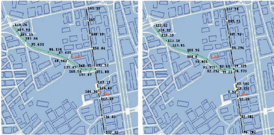
Fig. 1. a) Right map, required transmitted powers (dBm) of BS1 to block MSs; b) Left map required transmitted powers (dBm) of BS2 to block MSs.
